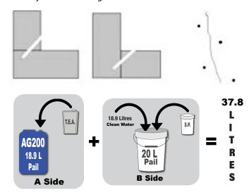
For curtain grouting, a grid pattern of appropriate size must be observed (typically 500mm x 500mm). This configuration should resemble a Dimond pattern.
